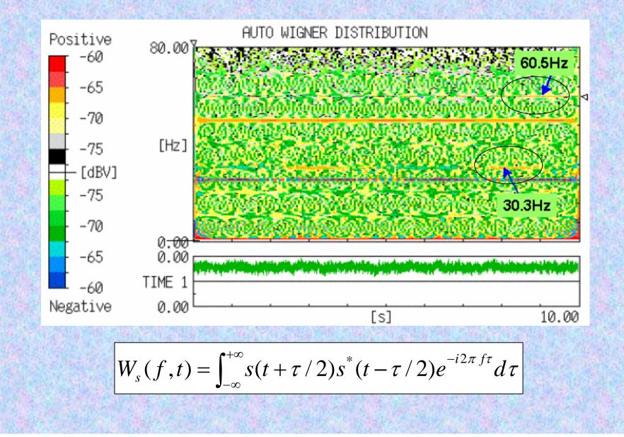
Frequencies of the signal detected, electric potentials measured at the output of the transducer and estimated amplitudes of gravitational waves from the Crab pulsar
